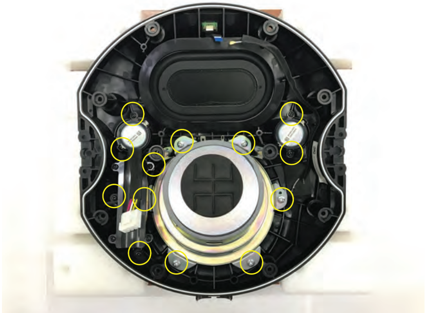
13: Remove battery box 3 screws and Tweeter/Woofer 10 screws
