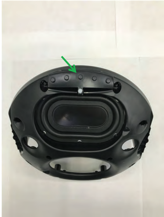
18: Remove handle and seal board
