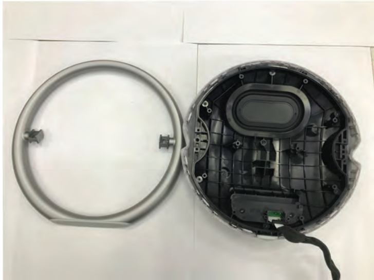
18: Remove handle and seal board
