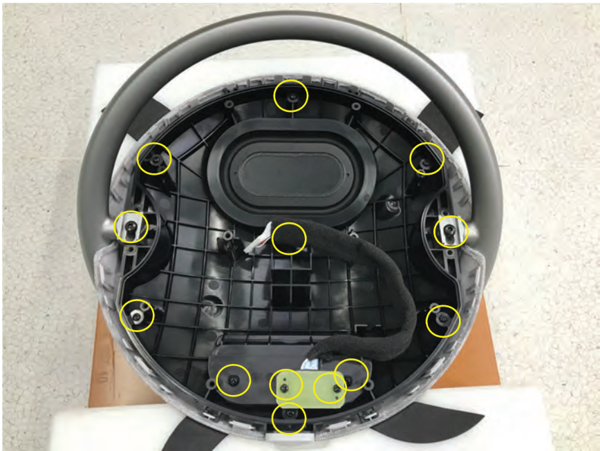
17: Remove handle 2 screws and grill fabric 11screws
